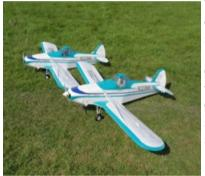
The final verdict being that it needed some down-thrust adding before it was capable of sustained flight.
