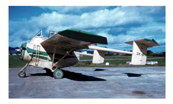
Photo of New Zealands P11 agricultural Airtruck, built from assorted Harvard aircraft parts. Circa 1959 This was used for spraying phosphate, note the cockpit above the fuselage hopper, this was to improve pilot survivability in a crash and the unusual independent tail booms to allow loading by hopper lorry. Although not pretty, it flew very well.
